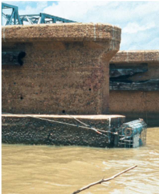
Turbidity logger in the Burdekin River Photo: M. Furnas, AIMS
