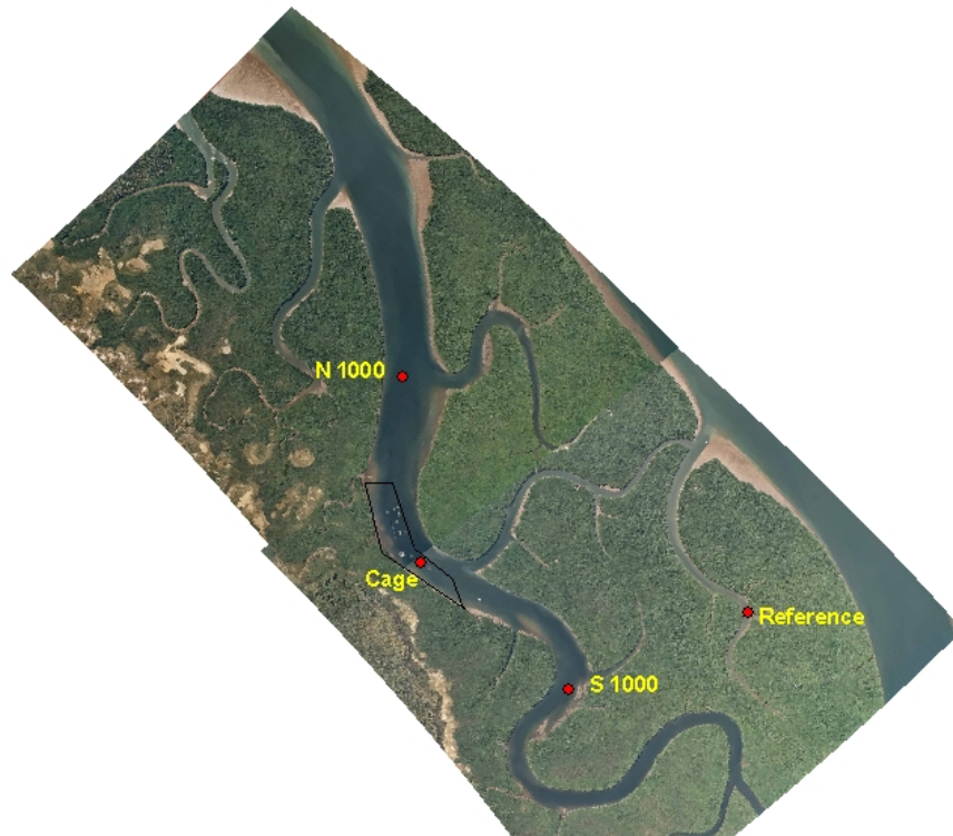
Figure 9: Sampling sites used for CTD profiles. The station notation indicates approximate distance (m) north or south of the Cage site. Note that the farm approval area indicated by the black polygon extends north of the “Cage” site by ~300m. The physical location of the “Cage” site differed between trips, as we sampled at the most heavily stocked cage, wherever that was within the farm.
