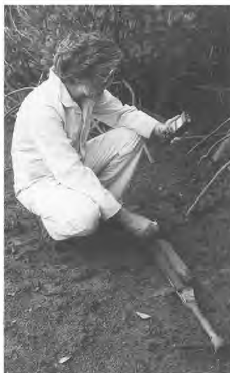
Figure 3.5 Taking readings from a core sample collected using a D-corer.
