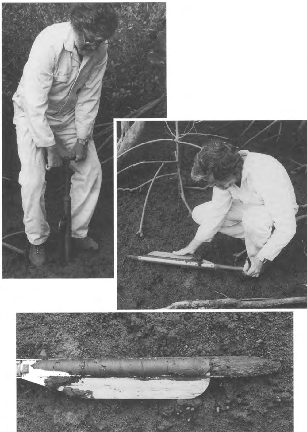
Figure 3.4 Taking a soil sample using a D-section corer.
