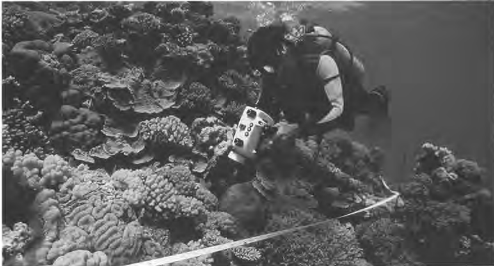
Figure AII.3 Diver recording the benthic community using a video camera.
