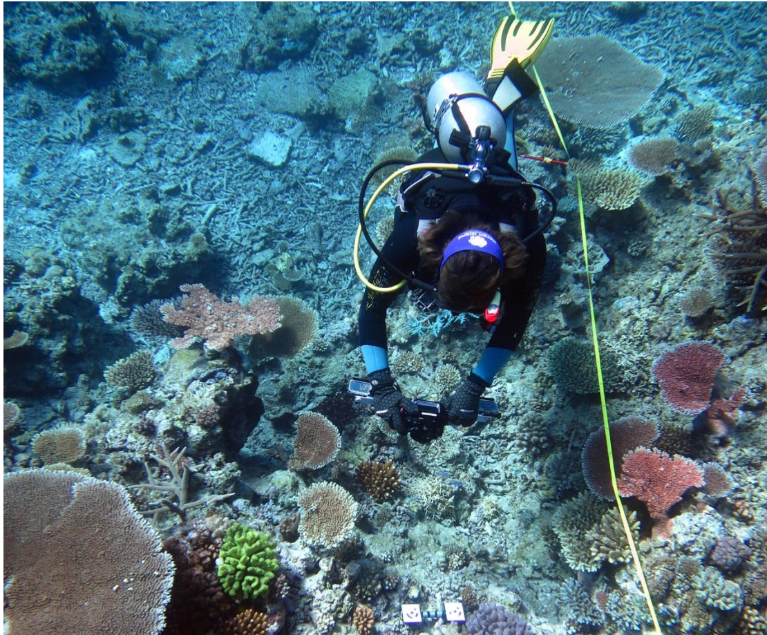
Figure 4: Diver collecting imagery along a transect for 3D reconstructions using a paired-arrangement of Go-Pro cameras set apart by 40cm. The picture also shows the Ground Control Markers (GCP) laid on the reef as a ground reference to scale the 3D reconstruction.
