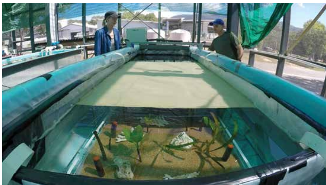
A large experimental tank with tide and wave action used in barrier experiments showing various receptors of oil (foreground), floating sorbents (olive) and the simulated oil spill (black at the rear of the tank).
