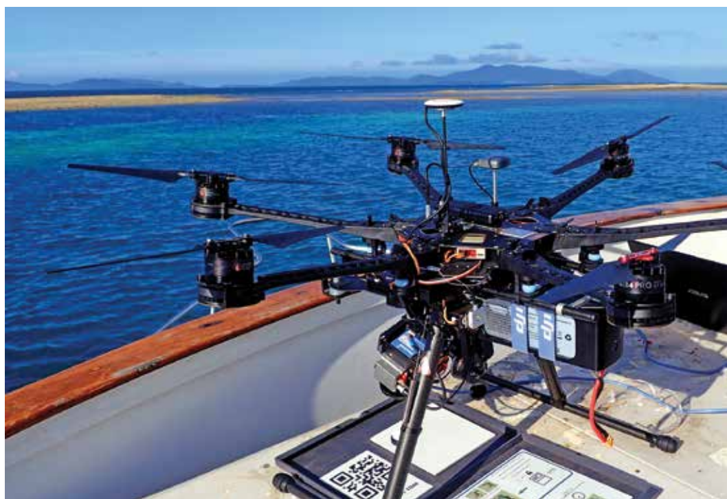
Aerial drones with hyperspectral cameras provide efficient assessments of shallow habitats.
