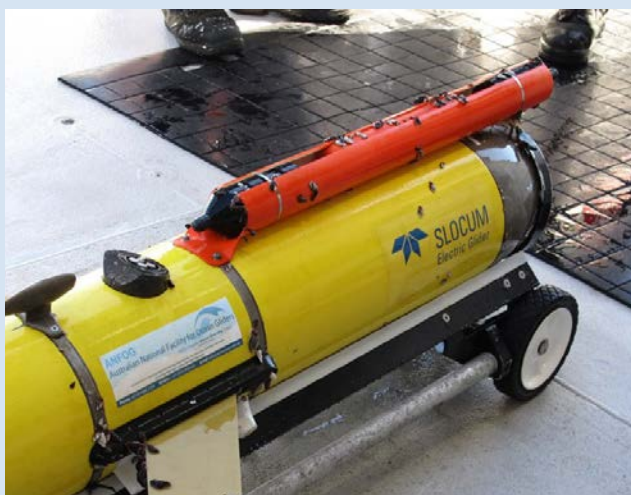
Left: glider deployed near Rowley Shoals recovered after ~ 1 month out on the Shelf sampling the water column and carrying a sound logger (orange) to record whale calls.
