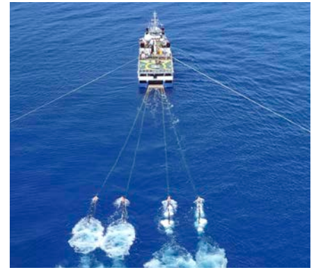
Above: BGP Explorer towing the air gun array for the North West Shoals to Shore Marine Noise experiment.
