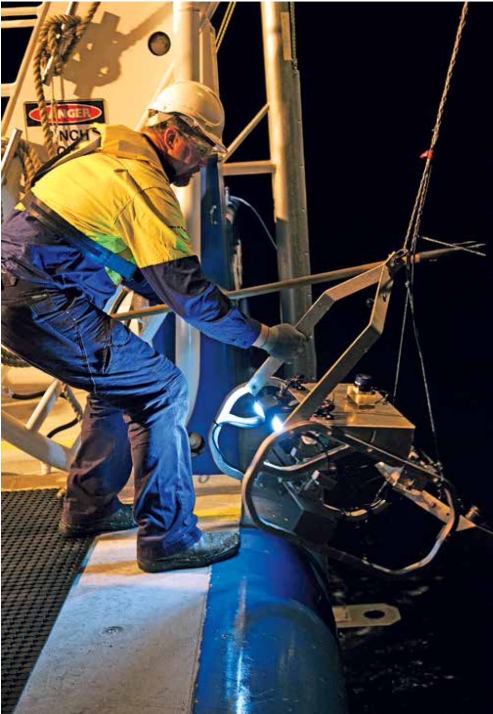
Towed video systems allow AIMS researchers to survey expansive tracts of seafloor quickly and accurately. Image: S. Clarke AIMS
