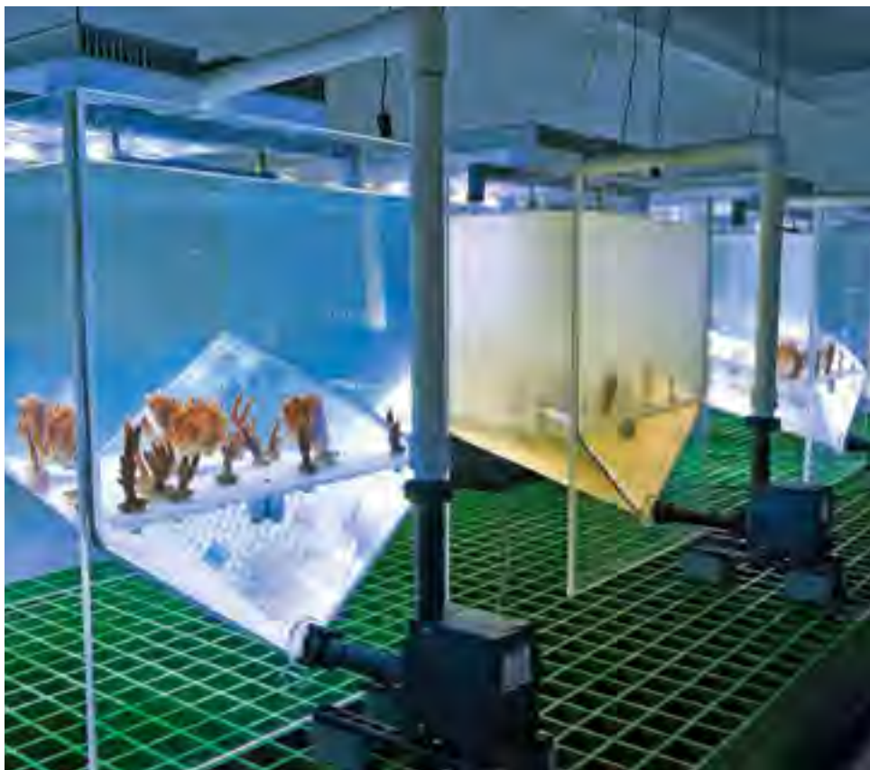
SeaSim will enable AIMS researchers to conduct experiments to assess the impact of pollutants and dredge spoil on tropical systems. Image: John DeRooy.
