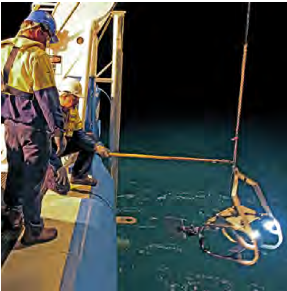
Towed video camera, being launched from the stern of RV Solander off NW Australia. Image: S. Clarke
