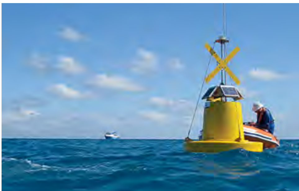
Instrument moorings along the GBR allow AIMS to capture detailed data about environmental conditions on the reef. Image: AIMS
