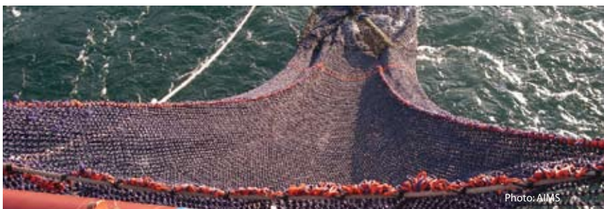
New benthic sled and cod net collects a sample of plants and animals living on the seabed which are used to help identify species recorded on video.
