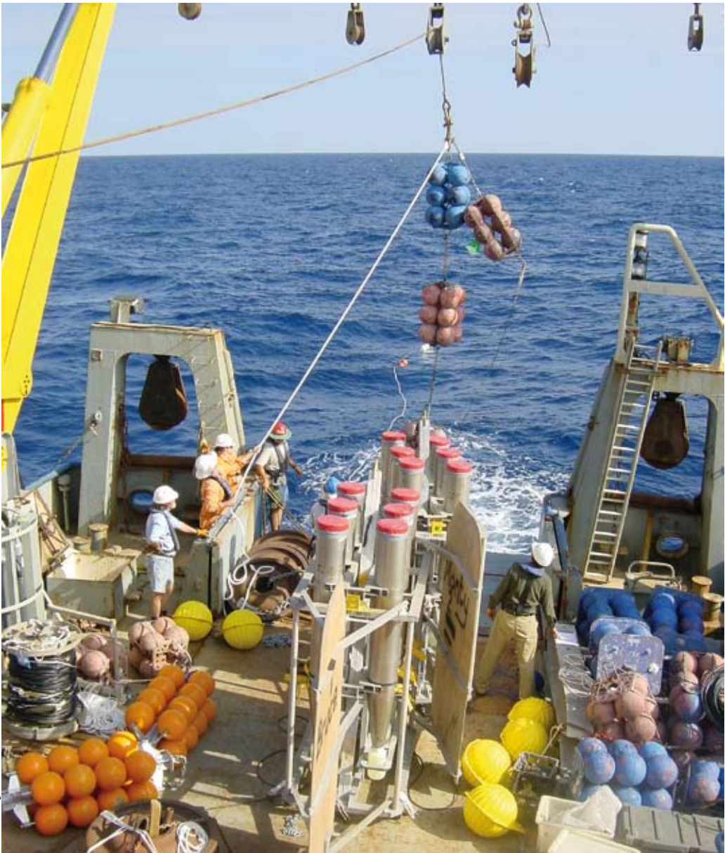
Deployment of sediment traps from the back deck of RV Southern Surveyor during a Timor Sea research cruise (see Highlight p 11).
