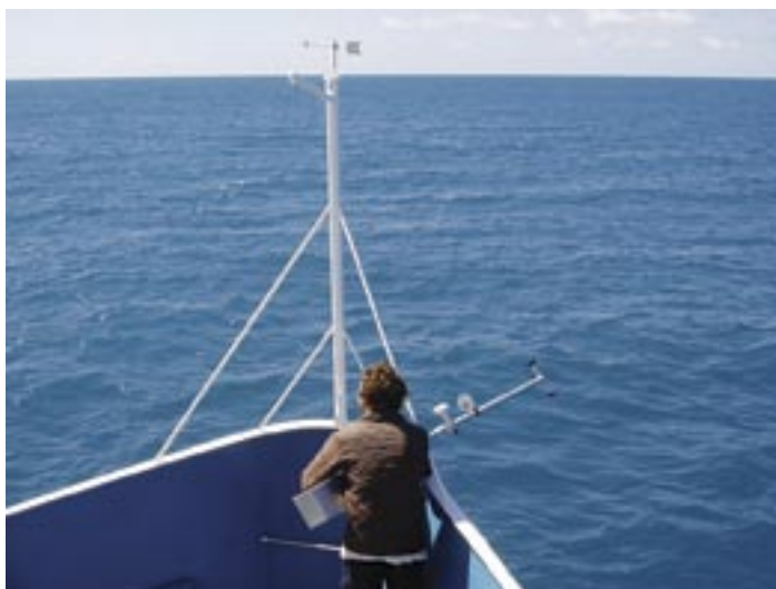
MEASURING OCEAN COLOUR SPECTRA FOR COMPARISON WITH SATELLITE DERIVED DATA
