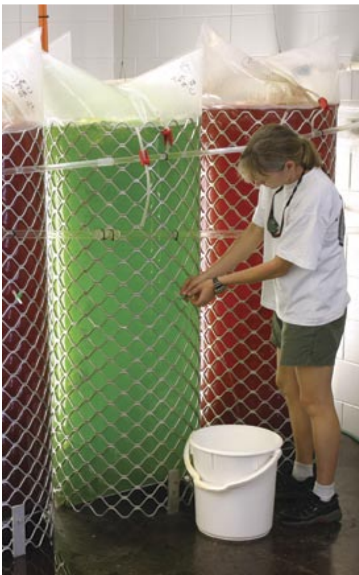
CONTINUOUS MICRO-ALGAL PRODUCTION SYSTEM IN THE AIMS TROPICAL AQUACULTURE FACILITY
