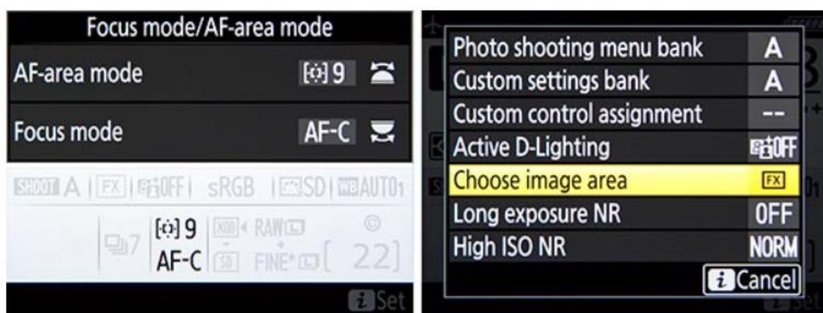
Figure 14 To change the AD-C symbol for AF-area mode –first ensure that the lever on the left front of the camera is on AF (NOT M), then press the button on the AF lever and use the scroll will to change to AF-area mode desired (AF-9).
