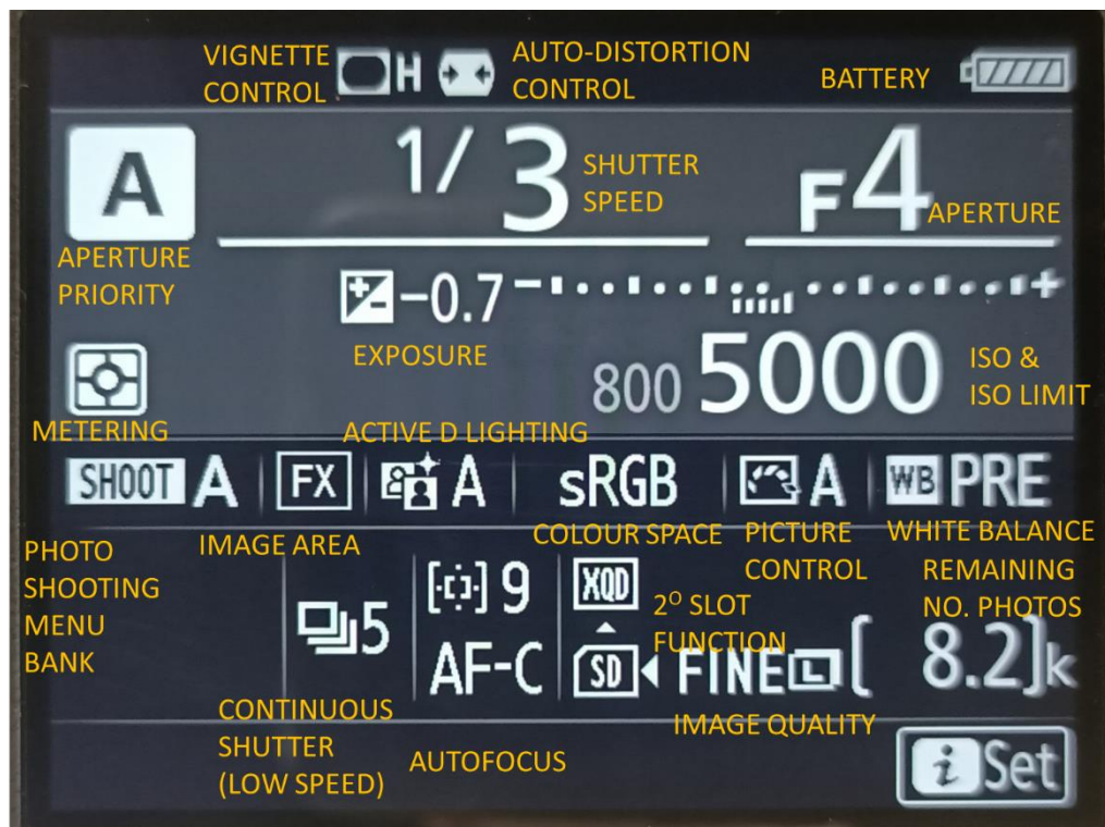
Figure 9. Photo of info display of Nikon D850 with recommended settings: (A) unlabelled, and; (B) labelled. Image: S.Gordon.
