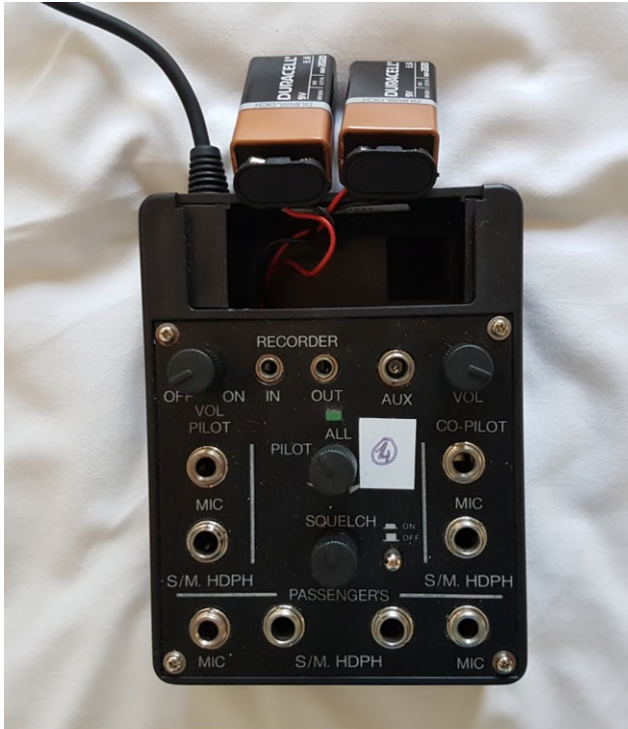
Figure 5. A 4-channel PA400S-ASC intercom box by Pilot Communications. There are 4 pairs of sockets to take headsets – designated as “pilot”, “co-pilot”, and two “passengers”. The audio recorder plugs into the “Out” socket
