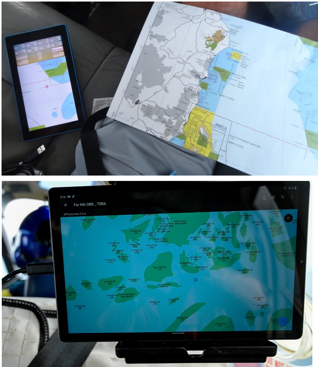
Figure 2. As used in 2017 and 2022, real-time navigational information is provided by an Android Lenovo tablet. Surveys are aided by running Memory Maps mapping software, and the AIMS coral bleaching app that operates within the ArcGIS Field Maps App, which includes GBR and Torres Straits reef features to guide flight path. The digital apps used in conjunction with hardcopies of the Reef Authority zoning maps to record bleaching observations, capture GPS locations of each data point and provide complete data records ready for analysis at the end of each flight through ArcGIS.
