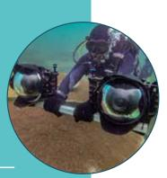
**ReefScan Diver** – the simplest configuration, comprising the ReefScan scientific payloads arranged for diver deployment. A basic example is the stereo machine-vision cameras with embedded Al for image analysis and a georeferencing system.
