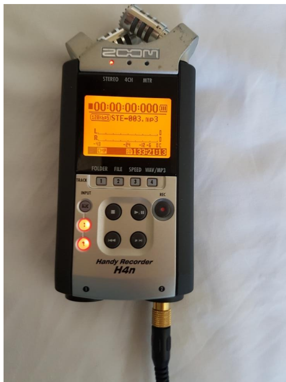
Figure 4. A four-channel Zoom Handy recorder H4n. The plug at the bottom right connects directly to the intercom box. Two intercom boxes can be plugged into the recorder at once. The stereo microphones on top of the recorder are only used when in autonomous mode
