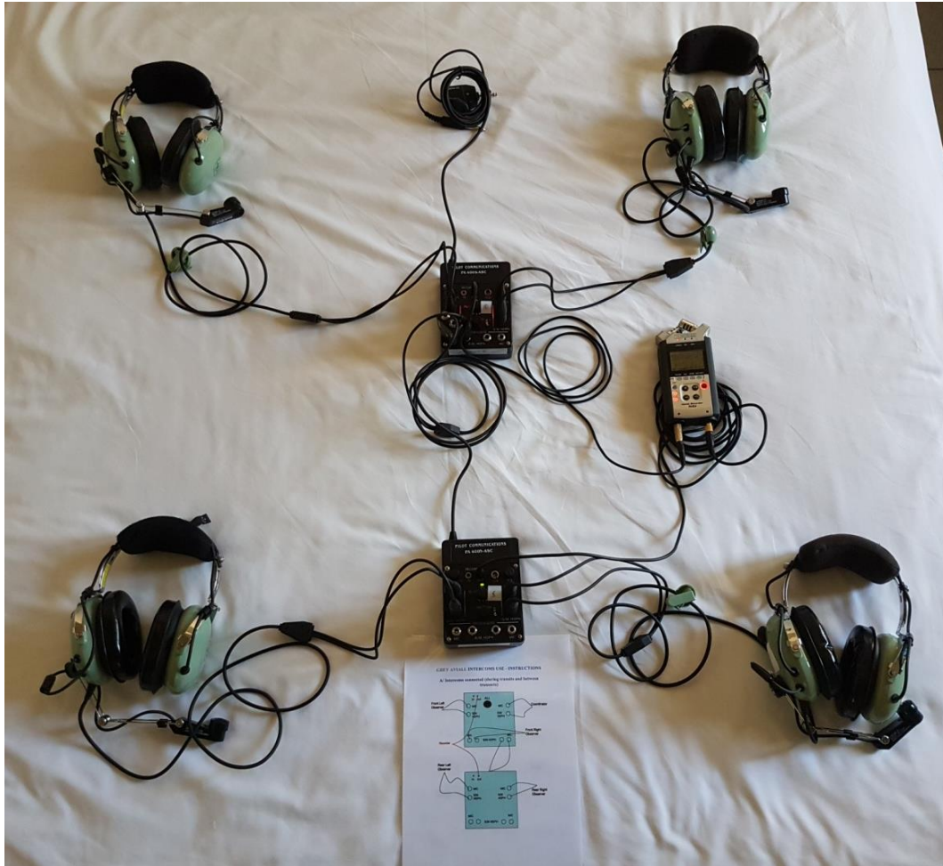
Figure 7. Four headsets plugged into two intercom boxes with a single audio recorder plugged into each intercom box. The two boxes are daisy chained via a set of connector leads which can plug into any socket-pair. The top intercom box can accommodate one more headset while the bottom intercom box can accommodate another two headsets. To use it so that all four (or seven) persons can talk to each other, the selector switch must be in the LEFT position.
