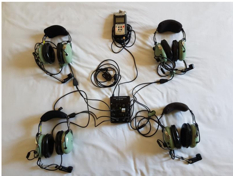
Figure 6. Four headsets plugged into a single intercom box with an audio recorder. To use it so that all four persons can talk to each other, the selector switch must be in the CENTRE position. Note that the daisy-chain plug-pair (top left of the intercom box) is left unplugged in this configuration.
