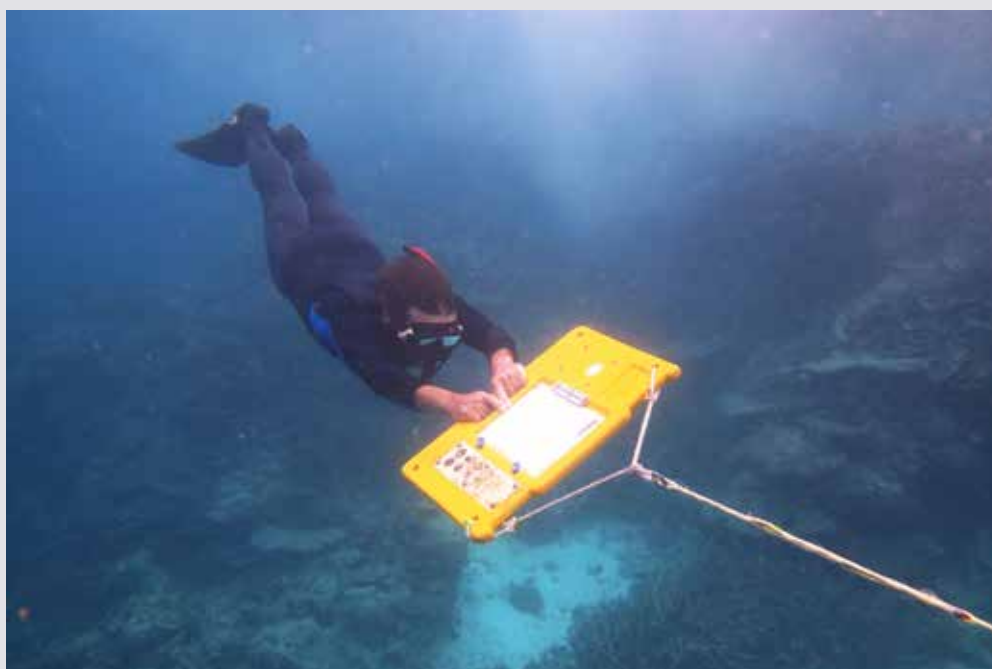
The manta tow method used by the Long-Term Monitoring Team provides estimates of coral cover and crown-of-thorns starfish populations around a reef. Image: LTMP
