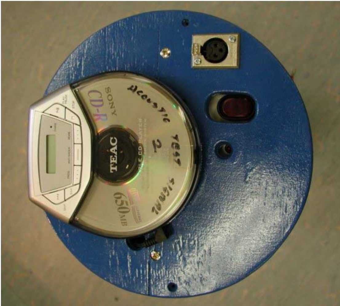
Figure 1. Upper view of acoustic system showing CD player (removed from waterproof housing).
