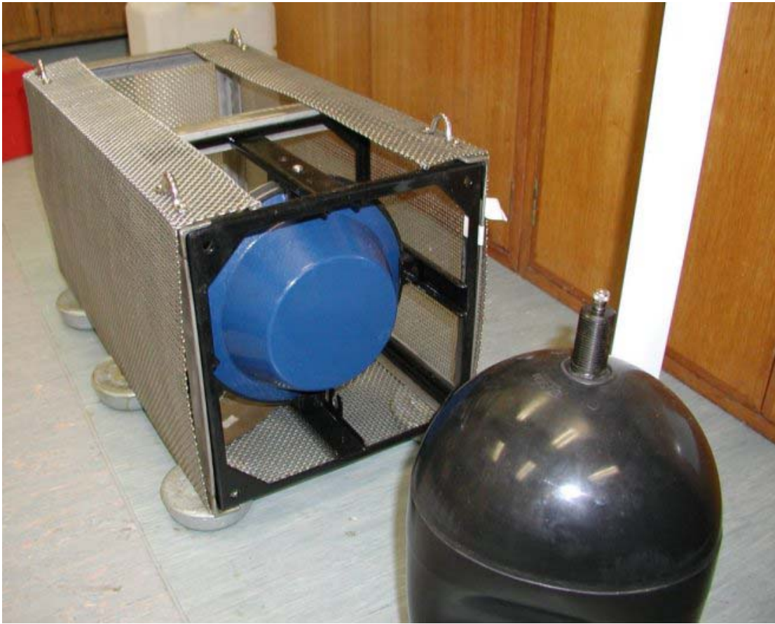
Figure 3. Underwater speaker, housing and compensation bladder
