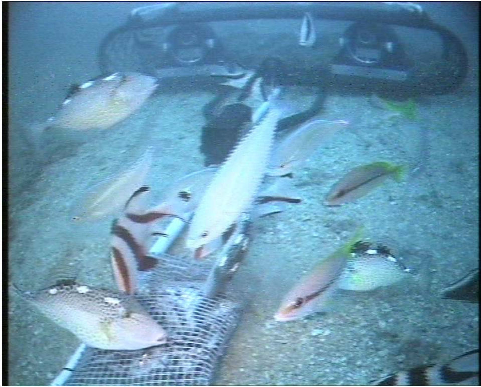
Figure 6. Stereo-BRUVS set on the seabed off Townsville. This unit was set on the seabed or hung from the mothership RV Cape Ferguson.
