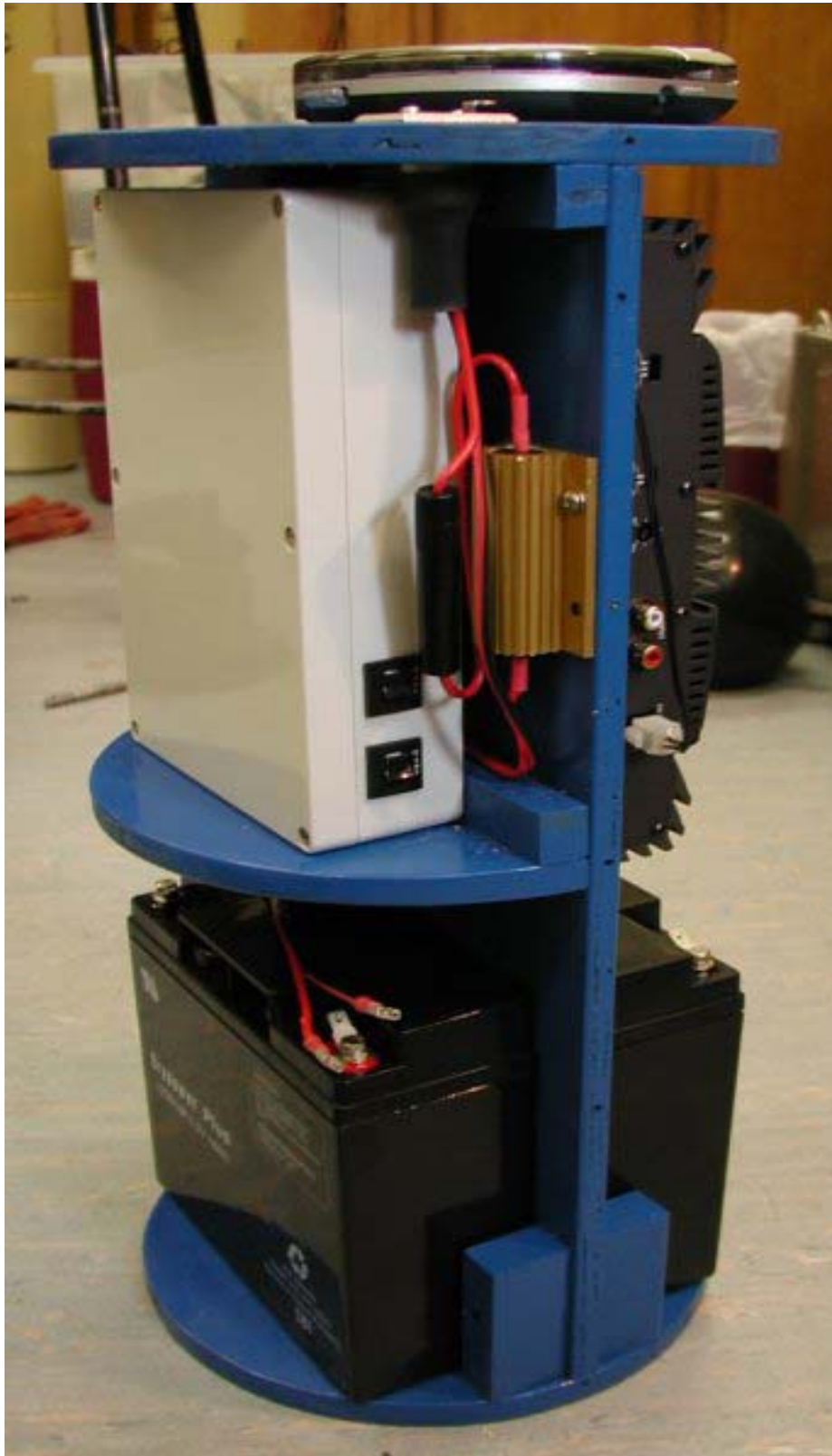
Figure 2. Side view of system showing amplifier and power source (removed from waterproof housing).
